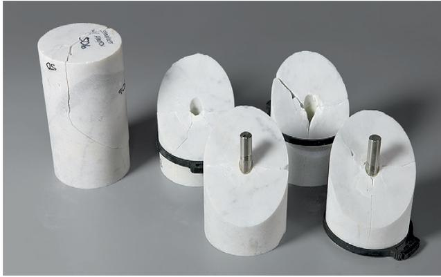
40. Upper and lower sections of three smooth-surface marble cylinders with fiberglass pins after testing. The marble was undamaged when the fiberglass pins were pushed to failure.
