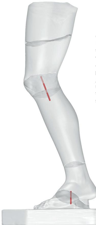
60a,b. Diagram showing the location and angles of the three fiberglass pins. One pin was inserted into the left knee, and one in each ankle. The pins were located where the joints were under compressive-shear force. Left: seen from the front. Right: the left leg seen from the side
