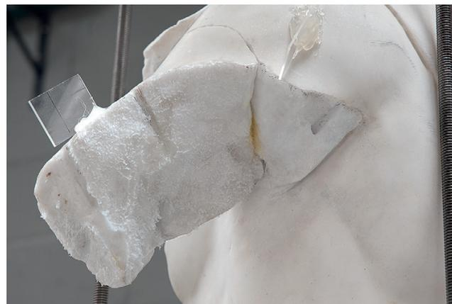
47. Torso of the *David* replica, showing the failed adhesive. Note the stringy, rough nature of the adhesive film, indicating that the overly thick layer had not fully set.
